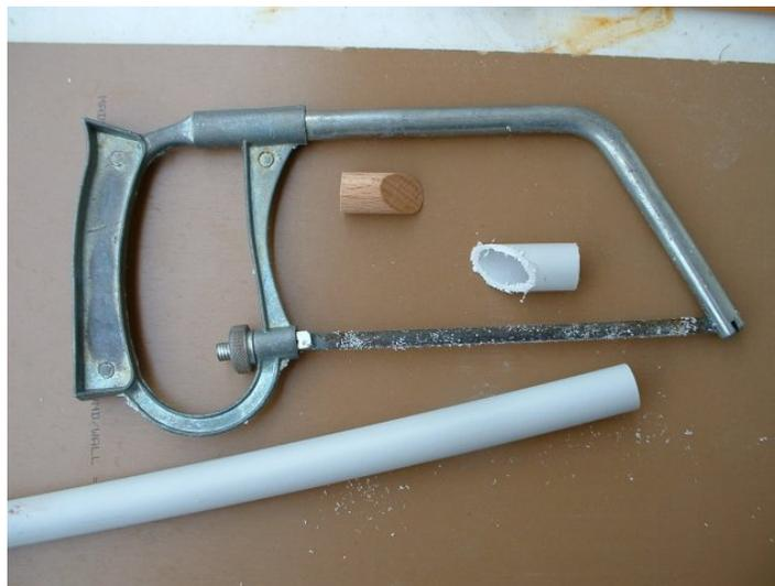
After sawing the PVC pieces to measure, make all ends, edges and sides smooth and well polished.
