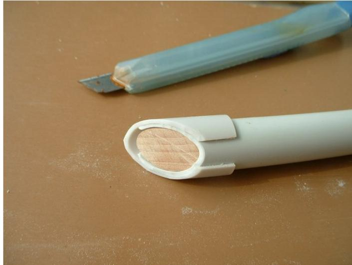
Peek through the windway: if the fipple block has the correct size, you should see a hairline of space just below the lip—say, **the thickness of two or three sheets of paper**. If you can't see this little space, the sound may be weak; sand the top of the fipple block as needed. *Beware not to sand too much*, or the whistle will consume more air and the second octave will sound harsh. As little as 1 mm may be too much!
