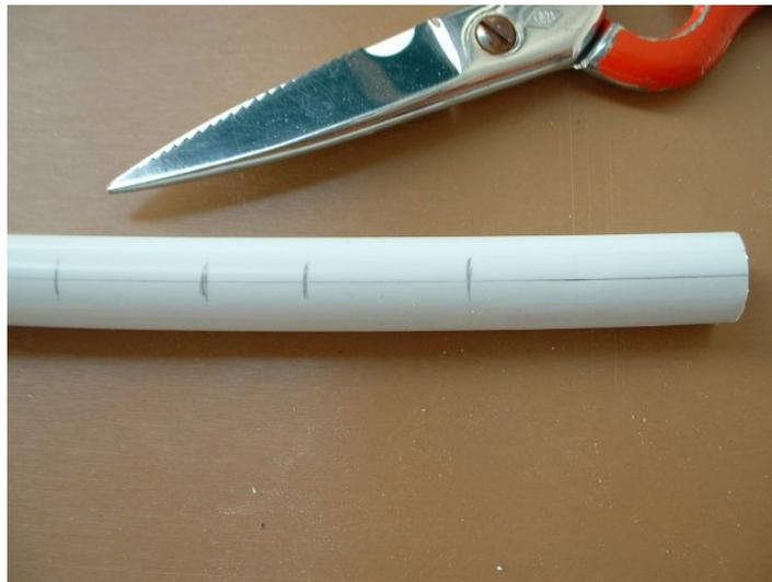
10. Bore the holes, starting from the bottom of the whistle. Twist the scissors tip to remove small amounts of PVC. **Work slowly.** Blow and check every note until it sounds OK; remember to check the notes on both octaves. The electronic tuner helps a lot here. You'll have to make a trade-off between the first and the second octave E; if the first is perfectly in tune, the second will be flat. Work out an acceptable hole diameter.
